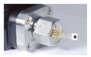
The short measurement window length effectively filters the long time constant variations in hardware and sensor response. Only short time constant, oxide surface adsorption contributes to the measurement. The end product is a robust thin film sensor design that provides the sensitivity and response time needed to effectively measure parts per billion levels of moisture.
