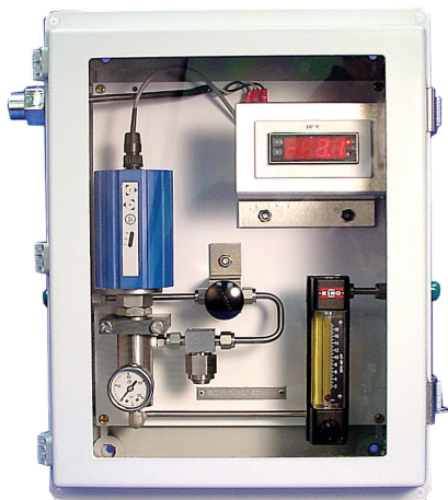
PSDA with CMX 1 transmitter in SS11 sample system
